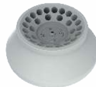
Cat. No. # LC02-L400-138 Capacity: 30 x 15 ml G-Force: 2391 x g
