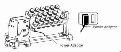
After connecting the power adaptor to back side of the device, switch the main power supply to "ON" & then switch the device on from the rear. Make sure that tubes are loaded properly before use.
